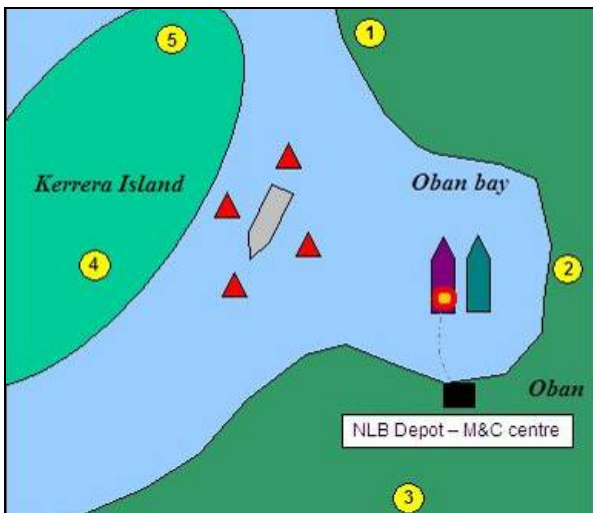
Figure 5: Part two of the demonstration scenario. Upon notification of the casualty, the GLAs used virtual AtoNs provided through AIS to mark the vessel (red triangles). In the meantime the GLAs vessel (purple) retrieves an emergency marker buoy from a second vessel.
